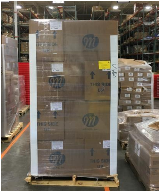
Improperly stacked pallet over 6'
